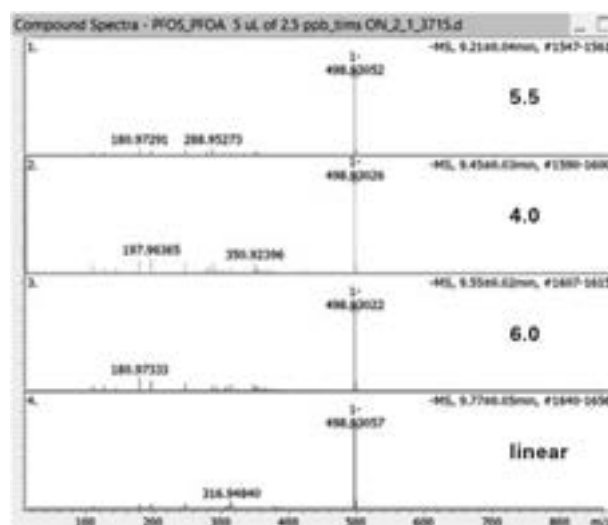
Figure 4. Mobility filtered mass spectra of each PFOS isomer within the studied sample. A 1:1 mixture of 10 mM sodium clusters and an Agilent tune mix solution was used for (external) mass and mobility calibration.
