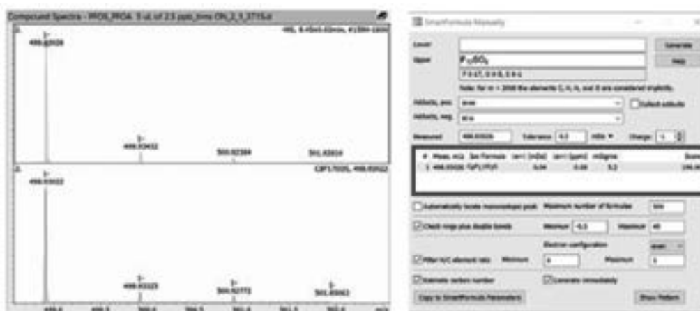
Figure 5. Mobility filtered mass spectra (target m/z range) for the perfluoro-4-methylheptane sulfonic acid (4), compared to theoretical (calculated) molecular weight and isotopic distribution of C_8HF_{17}O_3S . The mSigma value of 5.2 indicates a near-perfect fit. In this experiment, all mSigma values were <12 .
